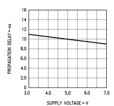
Figure 6. Typical Delay Characteristics (b)
