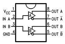
Figure 1. 8-Lead PDIP or CDIP or SOIC (Top View) See P or NAB0008A or D Package
