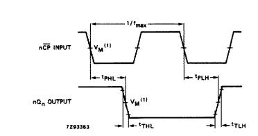
(1) HC :  $V_M$  = 50%;  $V_I$  = GND to  $V_{CC}$ . HCT:  $V_M$  = 1.3 V;  $V_I$  = GND to 3 V.
