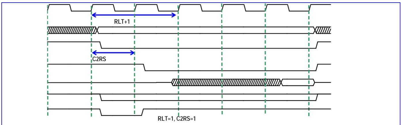
**Figure 17** Read Wait State Timing Diagram (ADVR=0)
