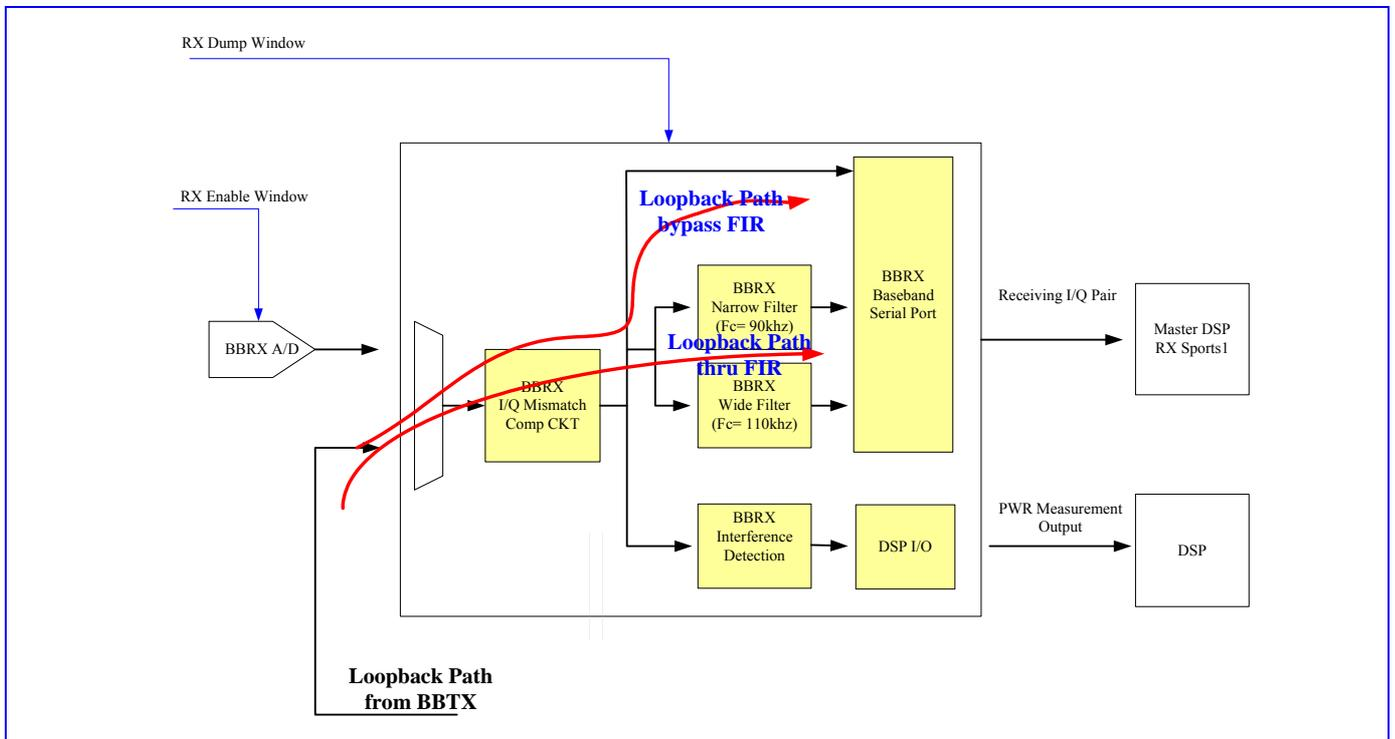
**Figure 53** Block diagram of RX path
