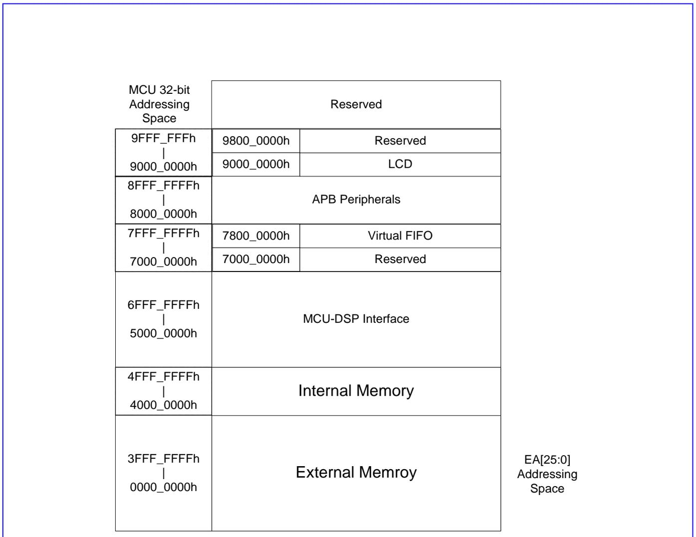
**Figure 6** The Memory Layout of MT6223
