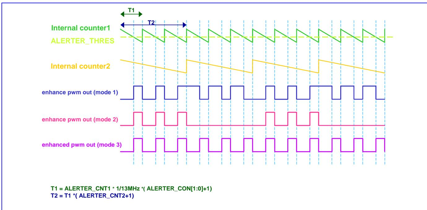
**Figure 21** Alerter Waveform
