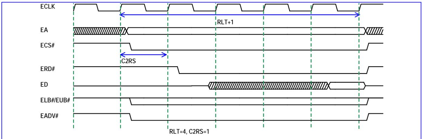
**Figure 16** Read Wait State Timing Diagram (ADVR=1)
