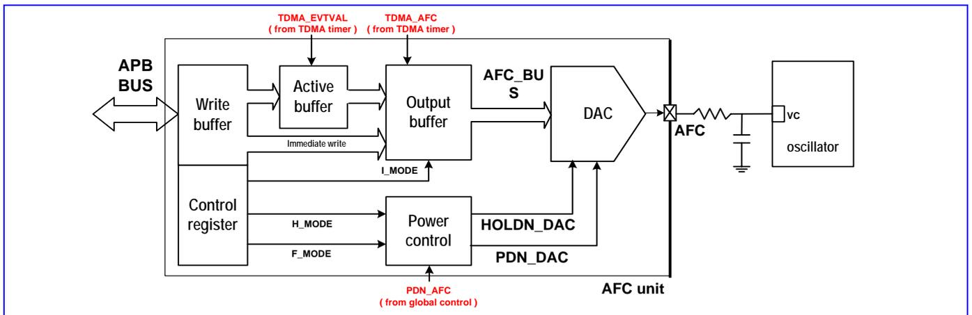
Figure 50 The block diagram of the AFC controller
