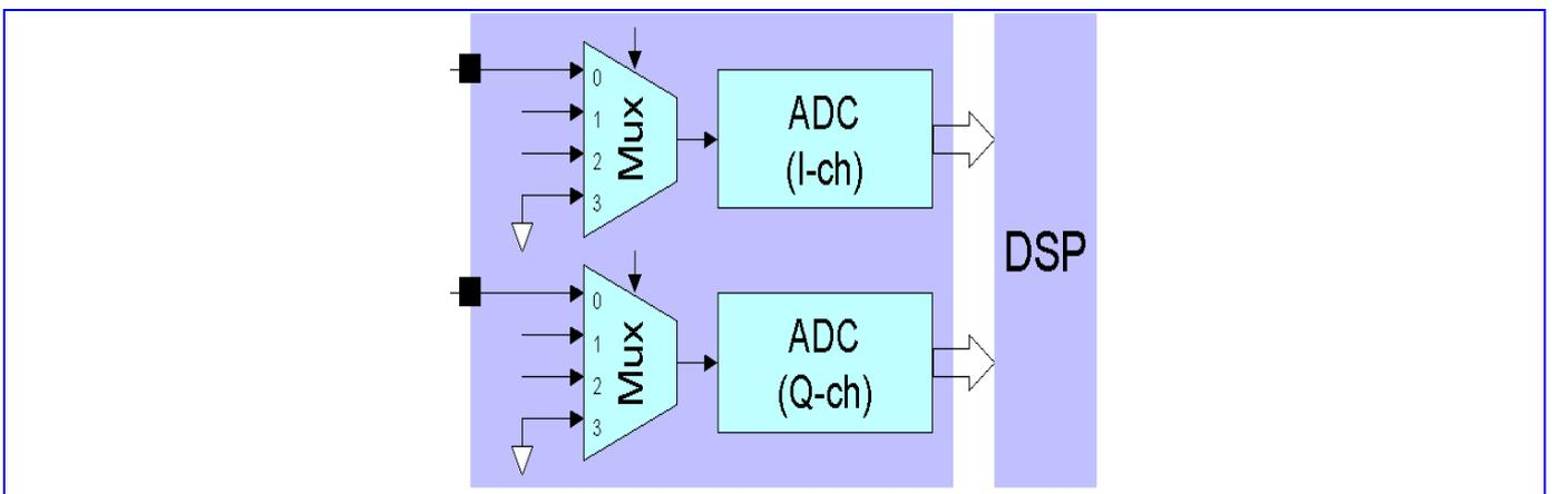
**Figure 79** Downlink ADC Offset Error Measurement
