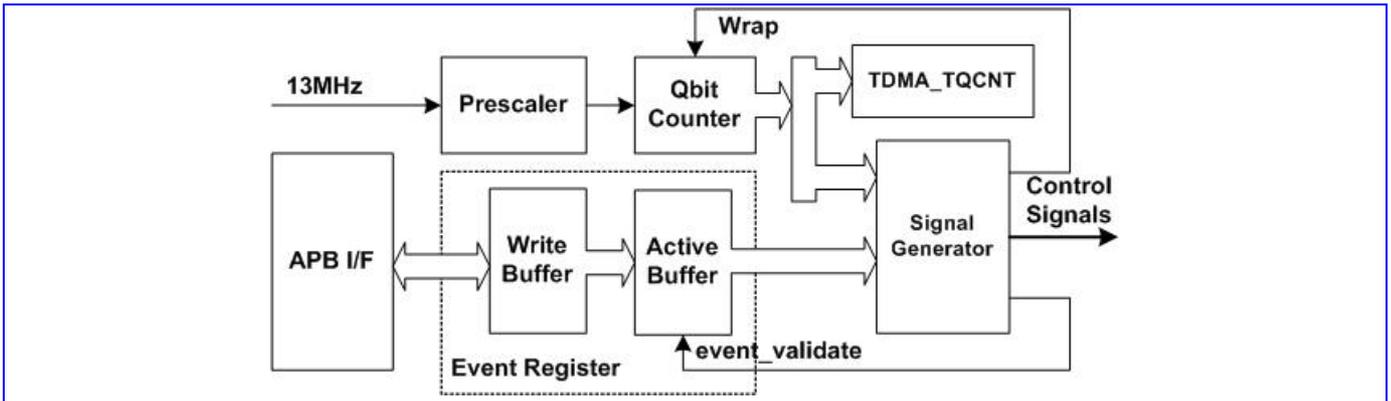
**Figure 65** The block diagram of TDMA timer
