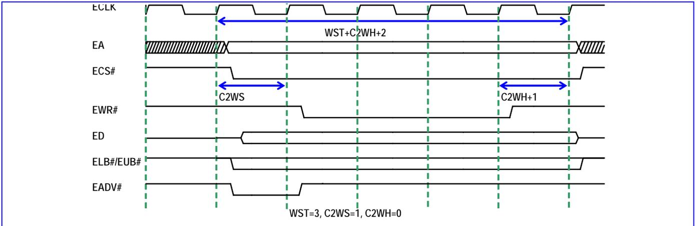
**Figure 19** Write Wait State Timing Diagram (ADVW=0)
