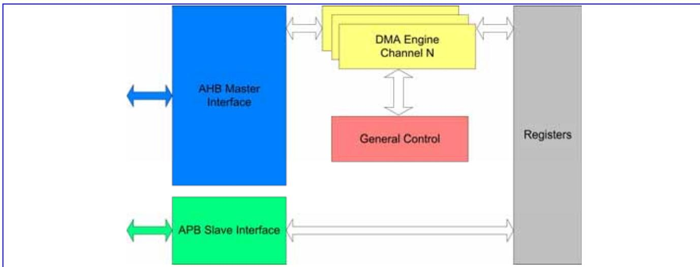
**Figure 9** Block Diagram of Direct memory Access Module
