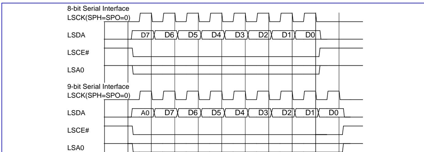
**Figure 27** LCD Interface Transfer Timing Diagram
