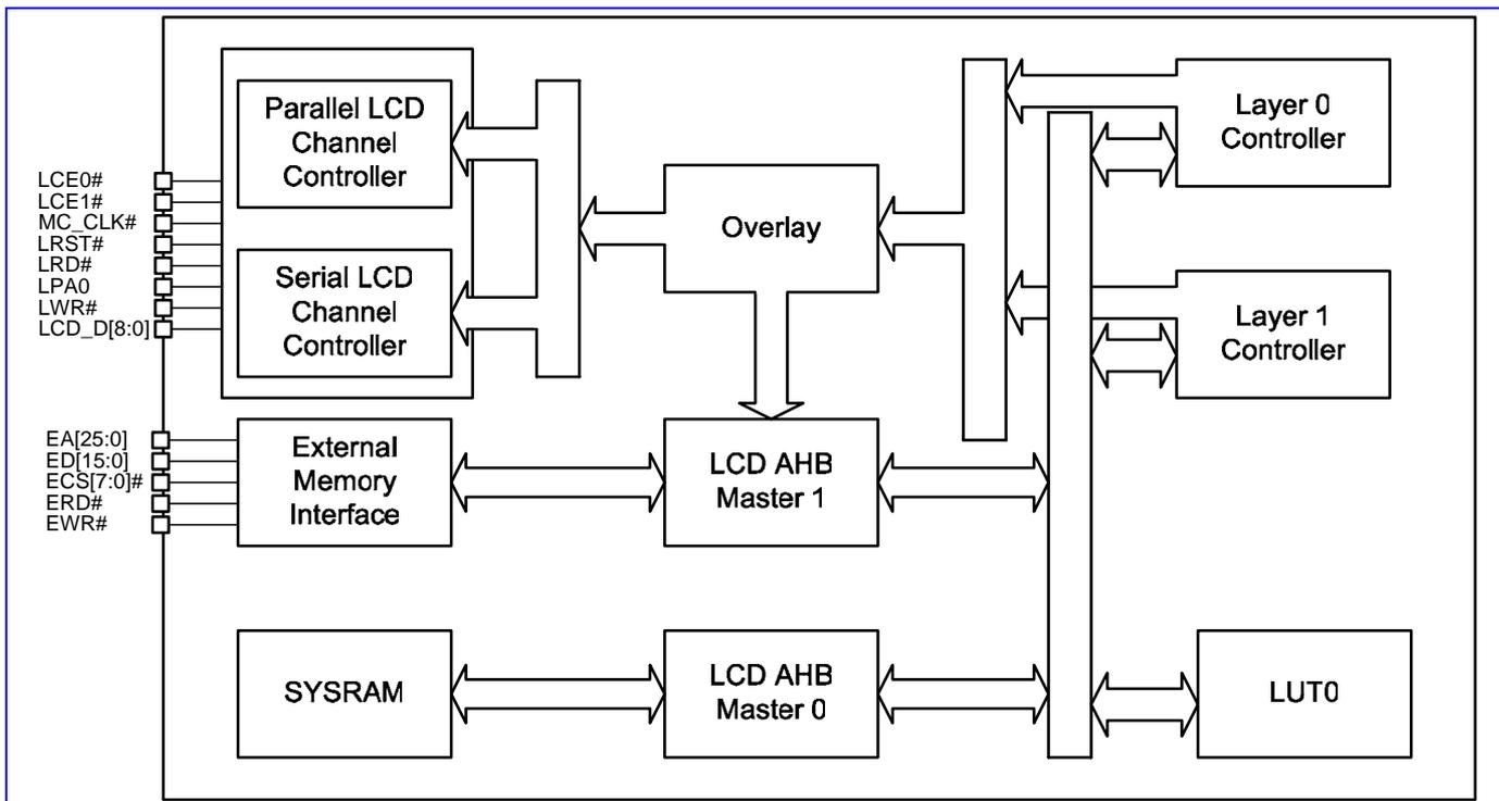
**Figure 26** LCD Interface Block Diagram
