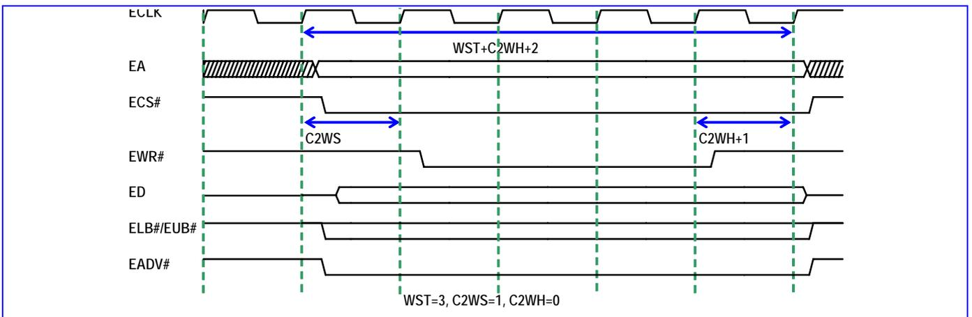
**Figure 18** Write Wait State Timing Diagram (ADVW=1)
