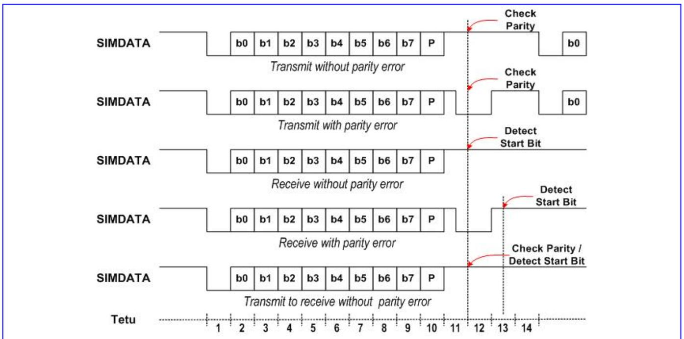
**Figure 24** SIM Interface Timing Diagram
