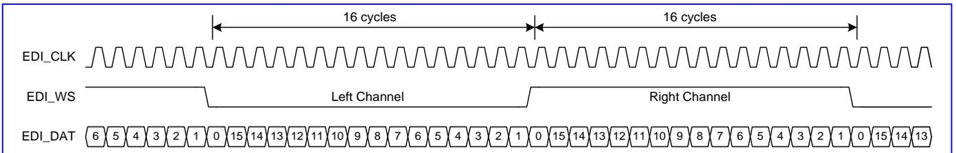
**Figure 63** Cycle count is 16 for I2S format.
