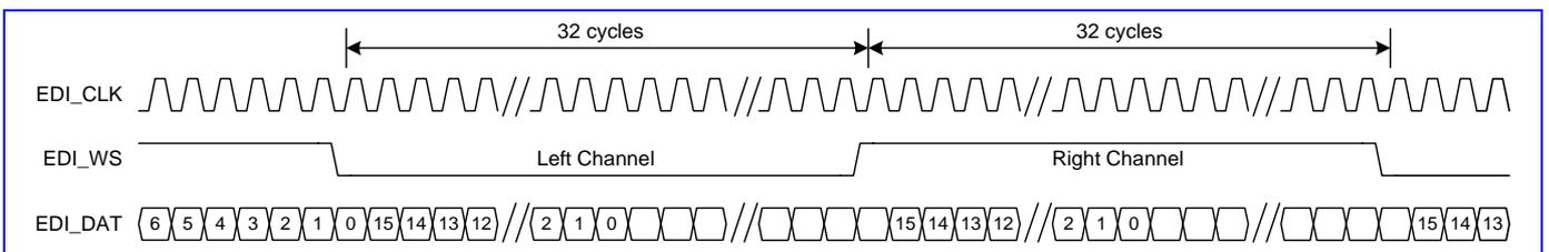
**Figure 64** Cycle count is 32 for I2S format.
