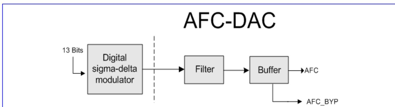
**Figure 74** Block diagram of AFC-DAC
