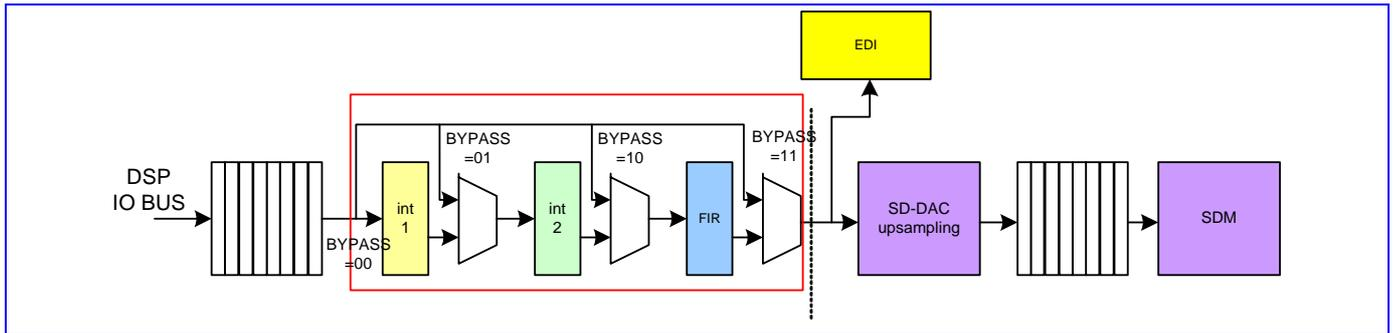
**Figure 62** Block diagram of the audio path.
