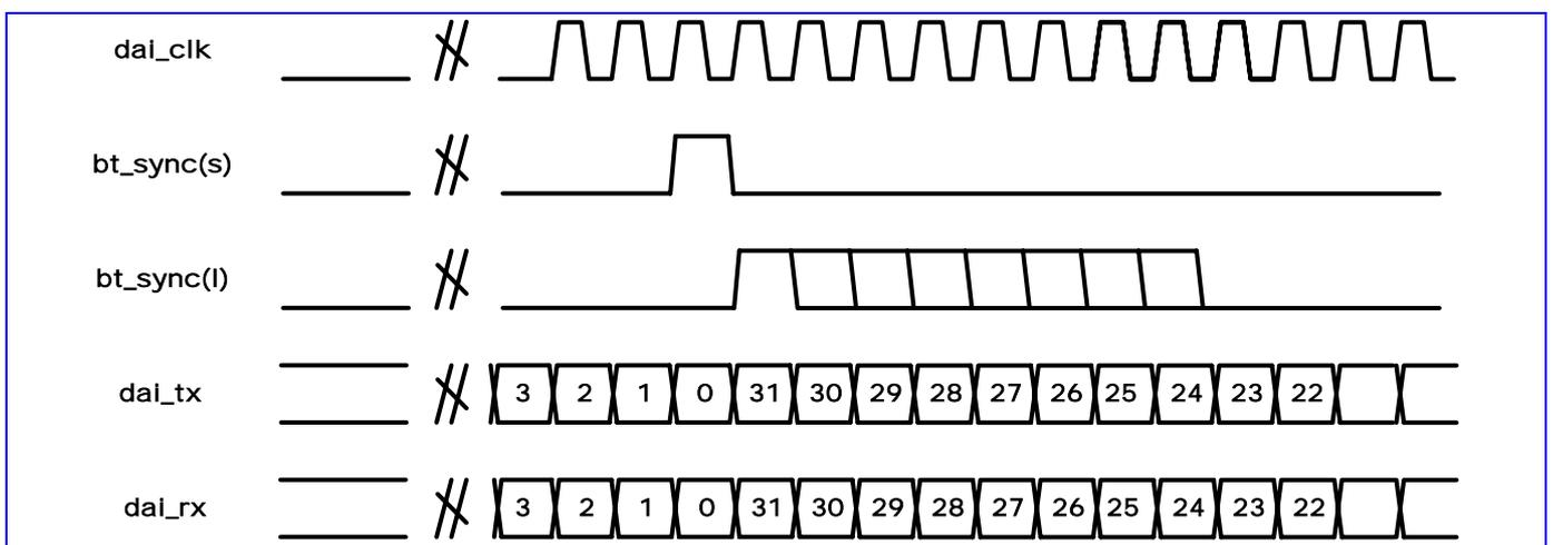
**Figure 58** Timing diagram of Bluetooth application
