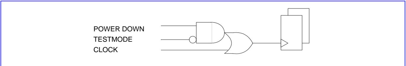
**Figure 69** Power Down Control at Block Level
