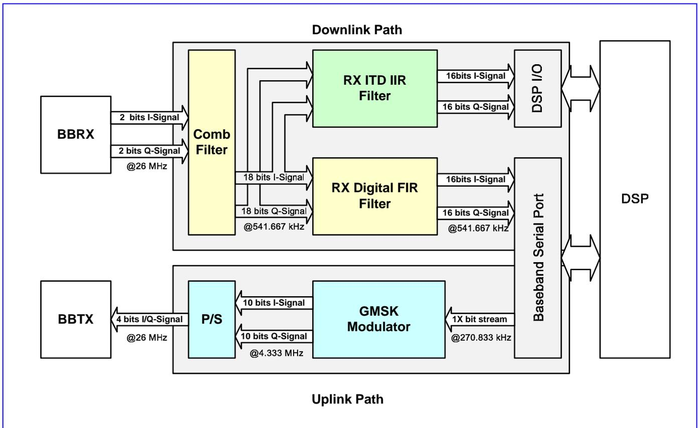
Figure 52 Block Diagram of Baseband Front End
