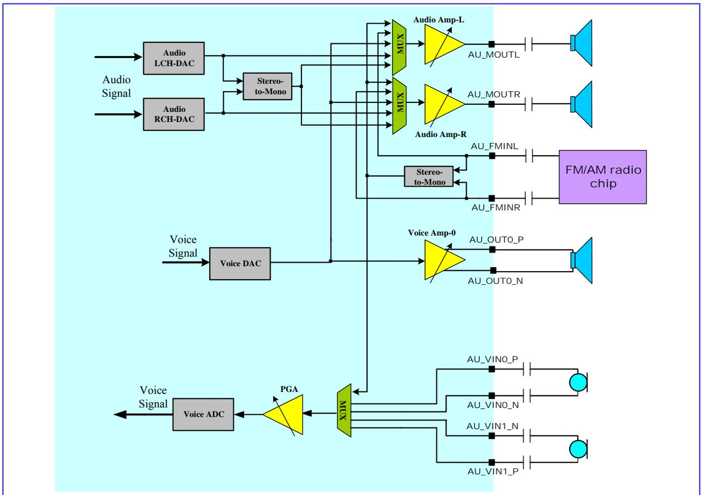
**Figure 75** Block diagram of audio mixed-signal blocks.
