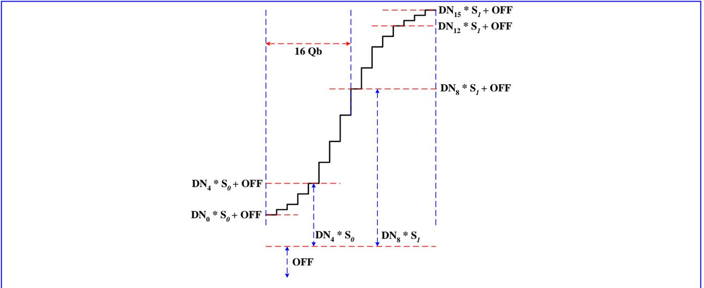
Figure 48 The timing diagram of the APC ramp.
