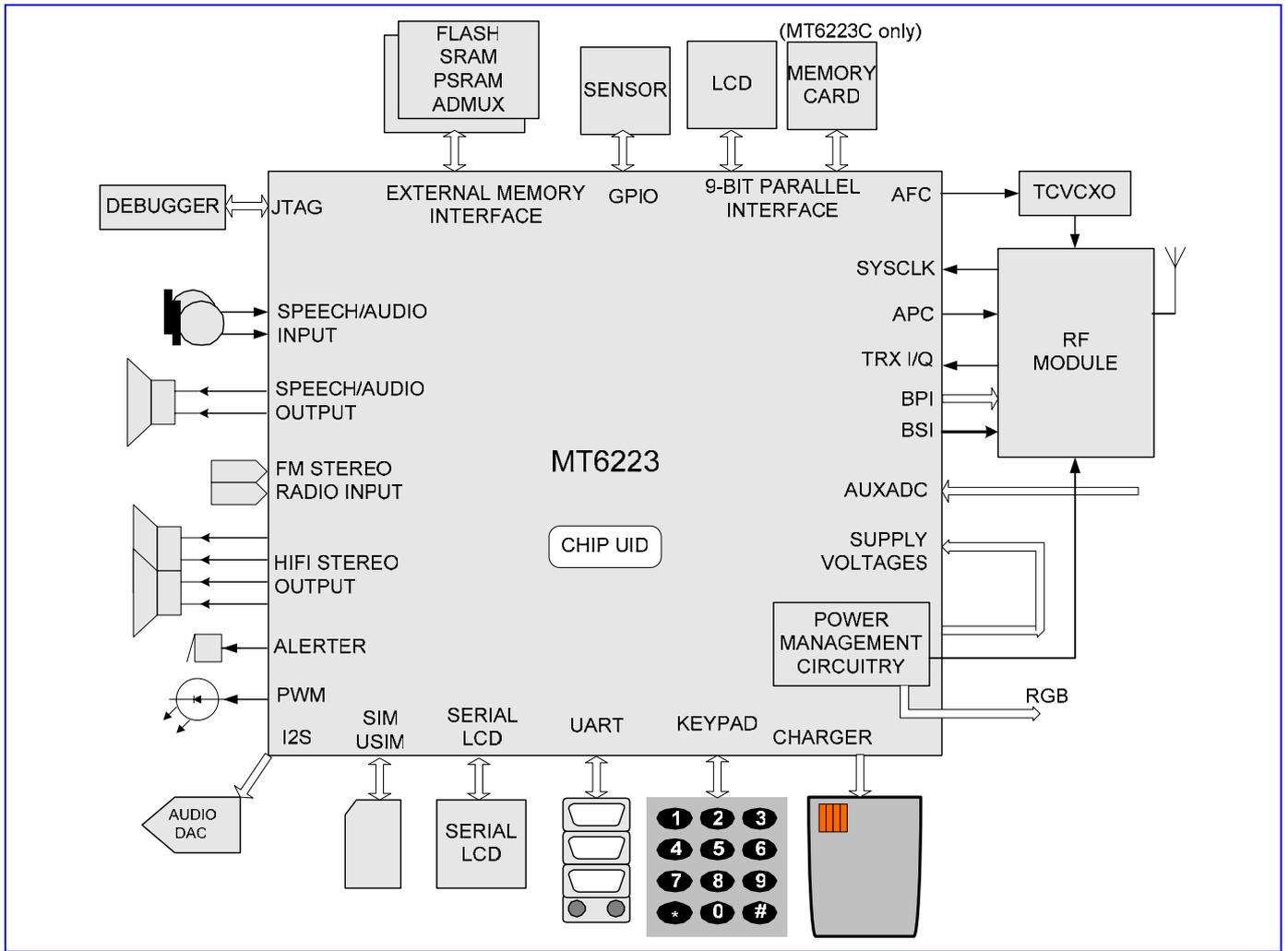
Figure 1 Typical application of MT6223.
