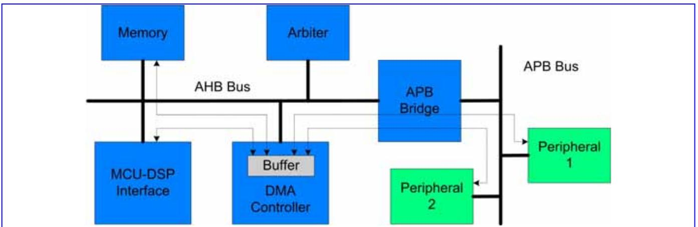
**Figure 8** Variety Data Paths of DMA Transfers
