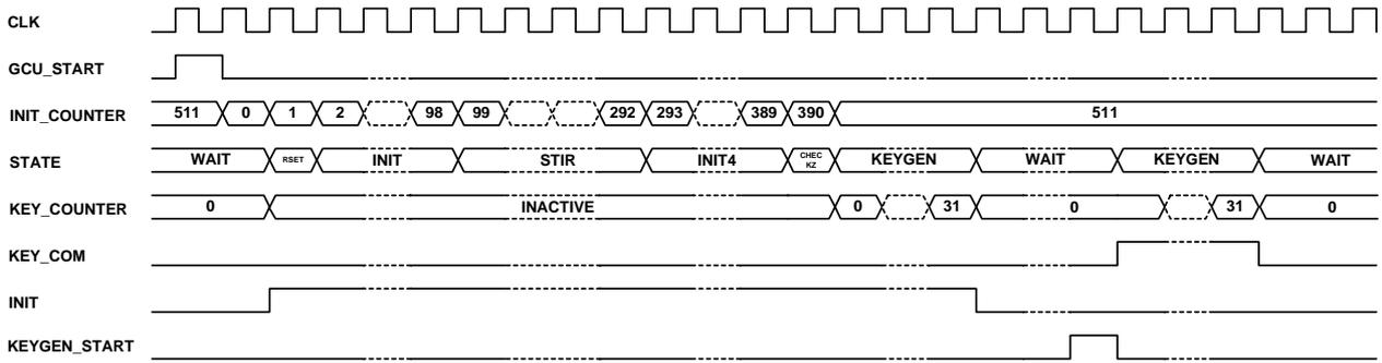
**Figure 33** The timing diagram of the GCU (in case of GEA2)
