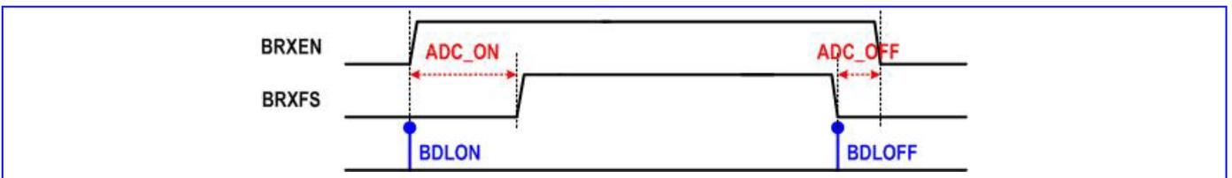
**Figure 66** The timing diagram of BRXEN and BRXFS
