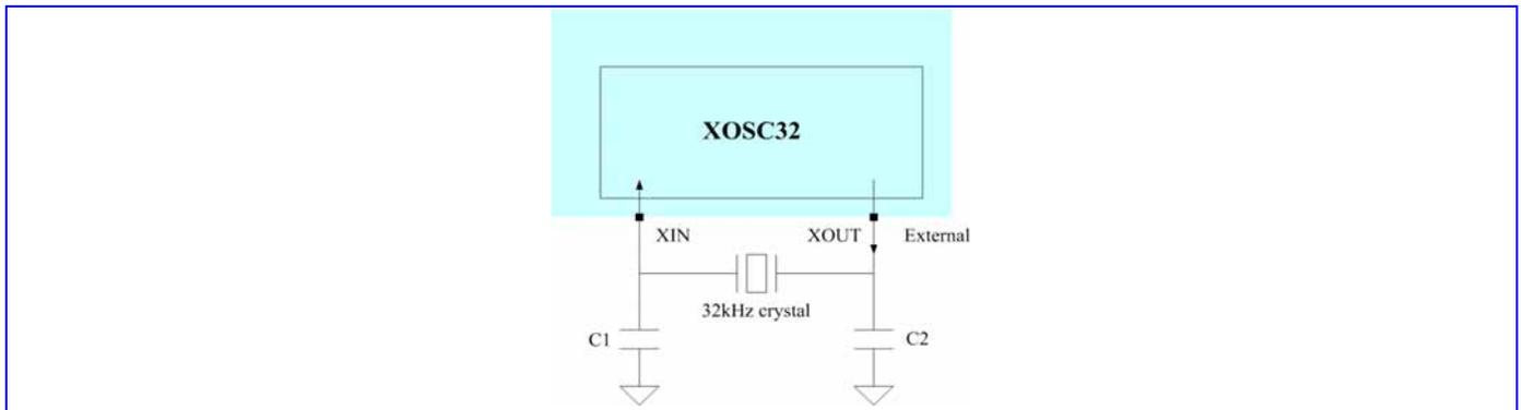
**Figure 77** Block diagram of XOSC32
