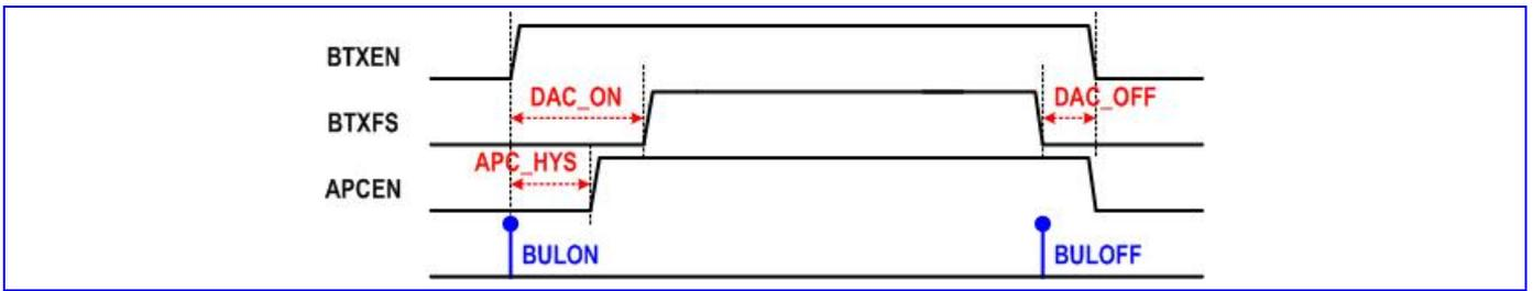
**Figure 67** The timing diagram of BTXEN and BTXFS
