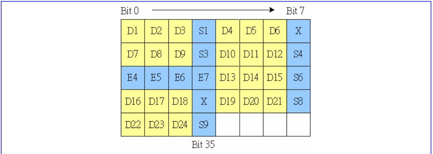
**Figure 38** data format conversion for 3.6k RA1
