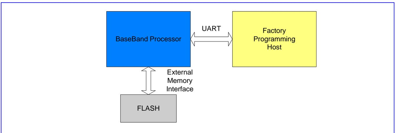
**Figure 7** System configuration required for factory programming
