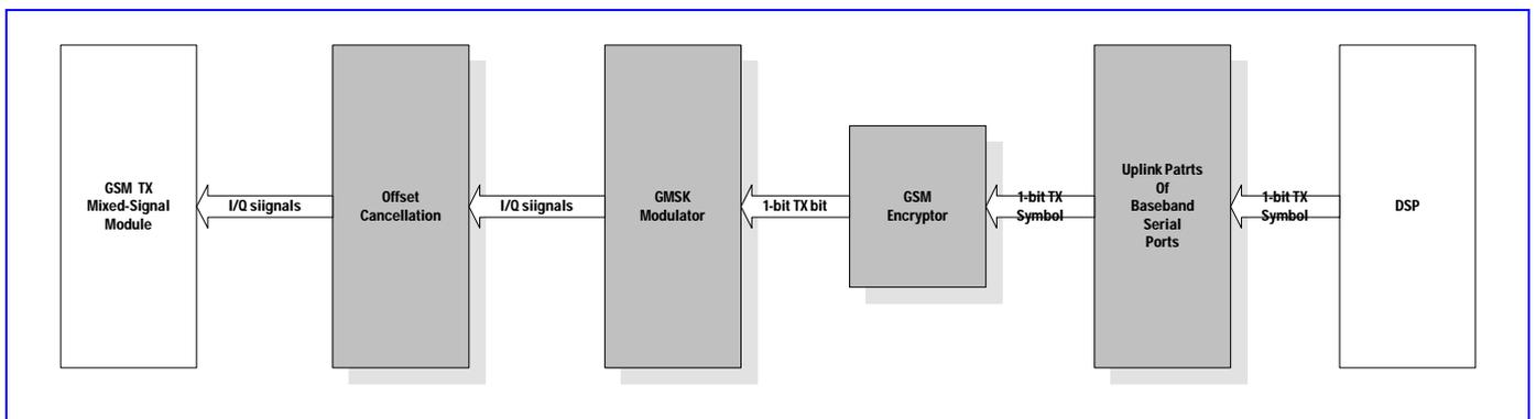
**Figure 55** Block Diagram of Uplink Path
