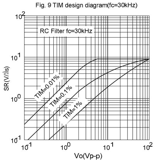
In Fig.8 The experimental results are shown for the 30W amplifier using the **HG TDA2030** as a driver and a low-cost complementary pair. A simple RC filter on the input of the amplifier to limit the maximum signal slope(SS) is an effective way to reduce TIM.
