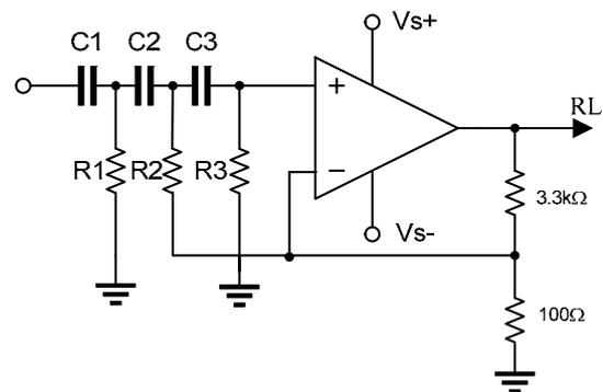
The components values calculated for  $f_c=900\text{Hz}$  using a Bessel 3rd Sallen and Key structure are:
